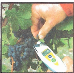
A BRIX refractometer performs a test on some grapes.
